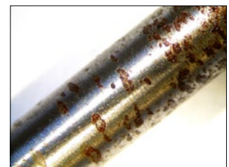
Corrosive fluids can cause premature stem failure.
